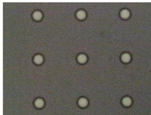
Figure 3: Microscope image (top down) of Pt vias after CMP.
