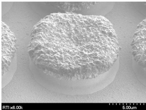
Figure 1: SEM micrograph of Pt via prior to CMP showing Pt plating overburden protruding above Si surface.
