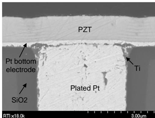
Figure 5. SEM cross section of a Pt via with PZT piezoelectric layer showing no cracking or degradation after 700°C anneal.
