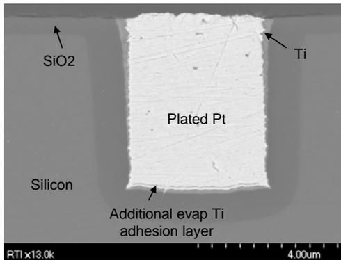
Figure 4. SEM cross section of Pt via after CMP processing.
