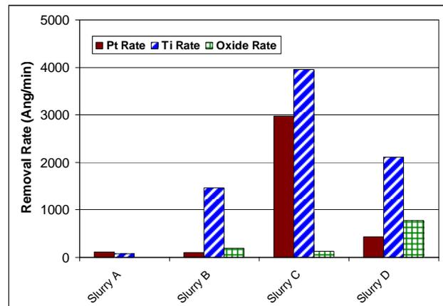
Figure 2: Graph of CMP removal rates for Pt, Ti and oxide for four different CMP slurries.
