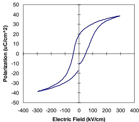
Figure 6. Ferroelectric polarization of the PZT film deposited above the plated Pt via test structures.
